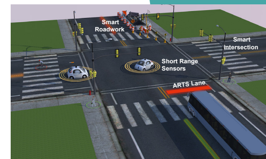
▲ Hybrid urban intersection adapted to the traffic of autonomous vehicles
