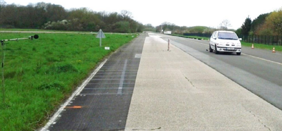
▲ Continuous measurement of embedded system rolling noise.
