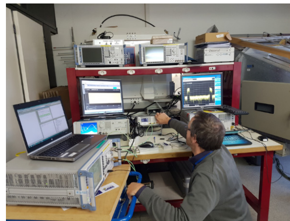
▲ Experiment to investigate the effects of a variety of electromagnetic attacks on the LTE system.
